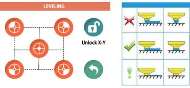
The distance between the nozzle and the platform is controlled to the height of 0.1-0.2mm, about the thickness of A4 paper. (Put on a A4 paper, feel the slight friction when you pull the paper)
